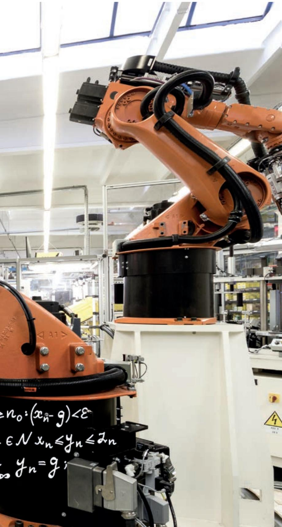
Use of a **high level of automation** has allowed the **assembly process** for commercial vehicle **calipers** to be fully **automated**.
